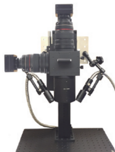
Side illumination and dual wavelength imaging
