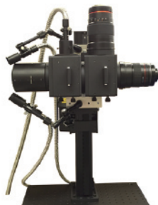
Epi-illumination and side illumination for dual wavelength imaging, 90 degrees rotation
