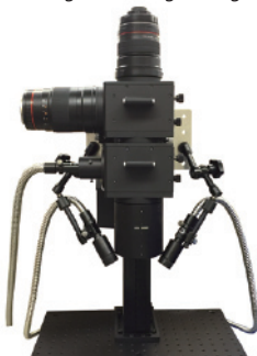
Epi-illumination and side illumination for dual wavelength imaging
